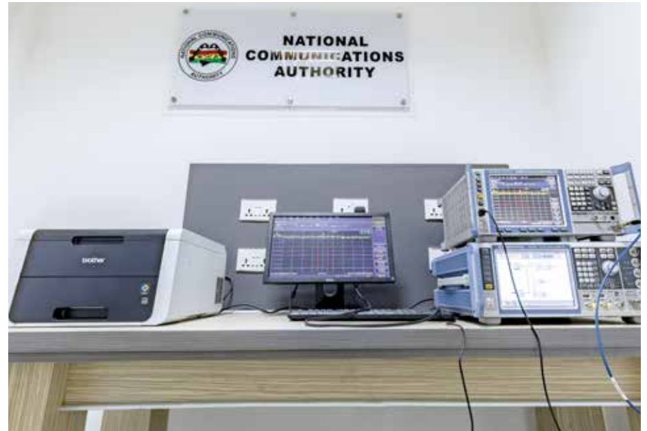
RF Signaling equipment at the NCA Type Approval Lab
