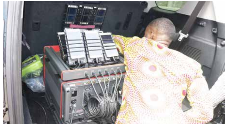
Staff of the NCA setting up the Drive Test equipment
