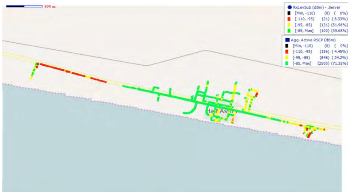
Remarks: Good coverage at Half Assini yet coverage improvement is required at the outskirts.
